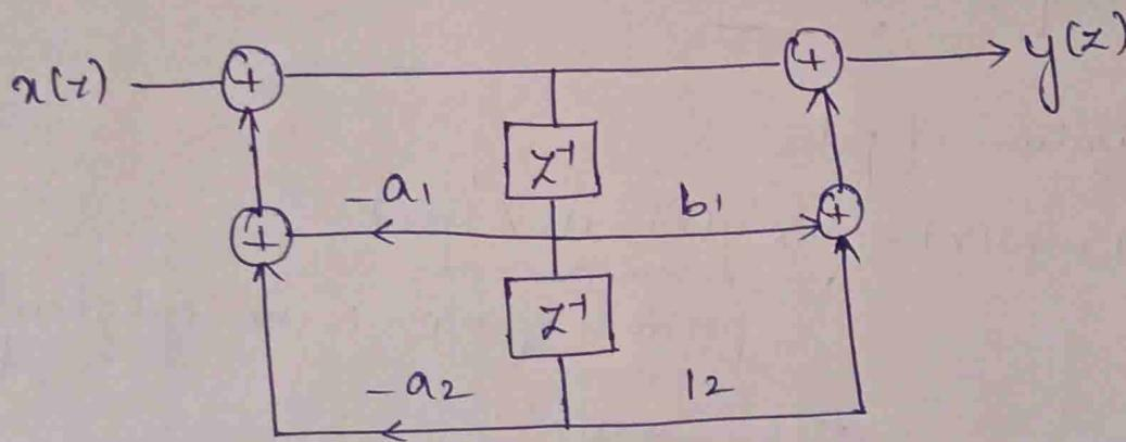
$w(n)$  is delayed by two unit delay block to produce  $w(n-1)$  hence can be replaced by one block.
