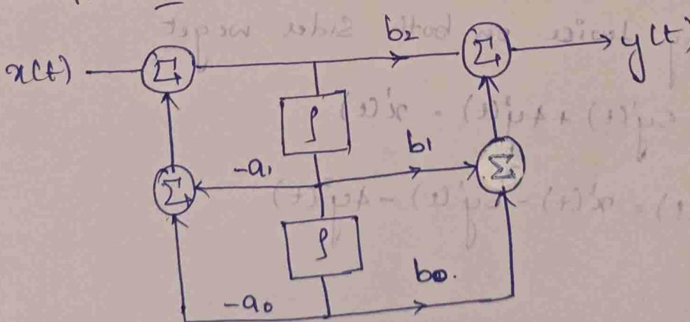
Q 1. By converting the differential equation to integral equation, draw direct form I and direct form II implementation for the system.
