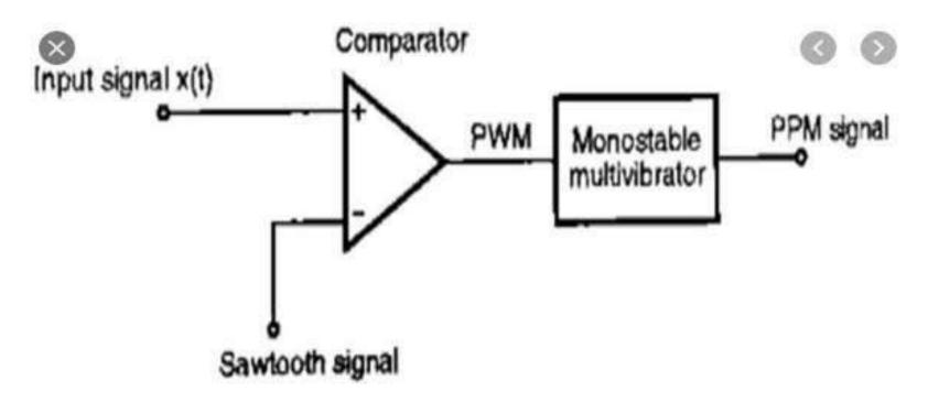
A sawtooth generator generates a sawtooth signal of frequency fs.
