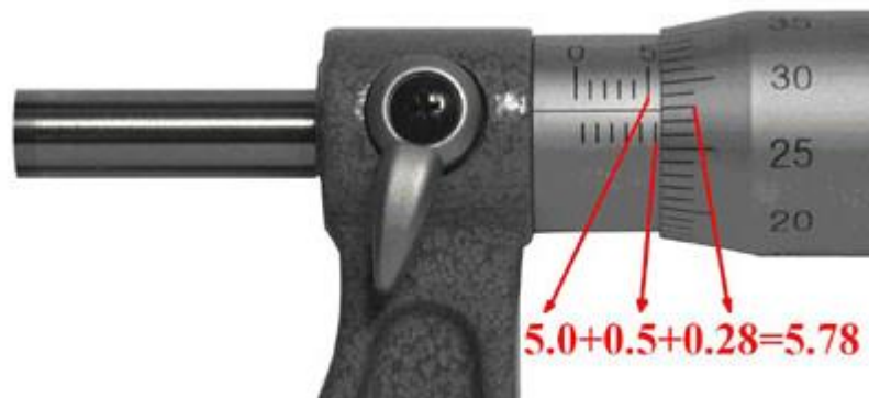
Micrometer thimble reading 5.78mm
