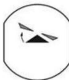
(e) Fly right command. Fly the aircraft to right to satisfy command bar
