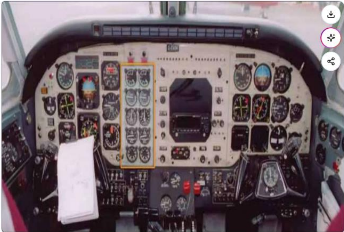
Figure 10-7. An engine instrumentation located in the middle of the instrument panel is shared by the pilot and co-pilot.
