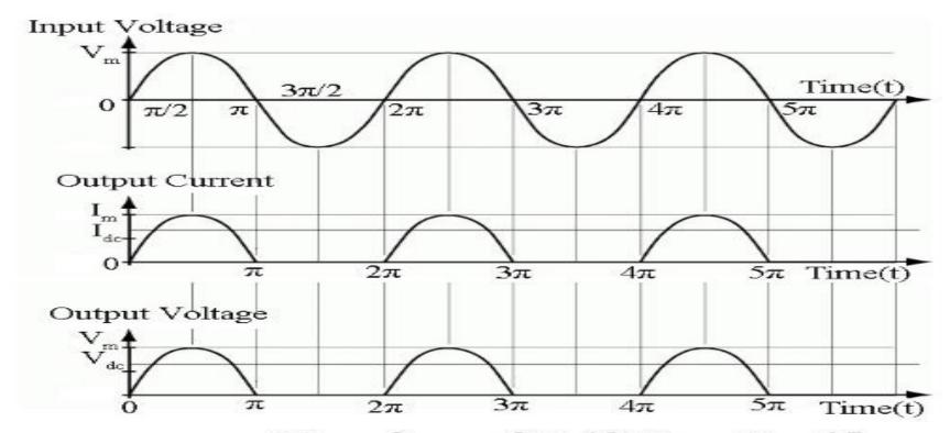
Waveform of Half Wave Rectifier
