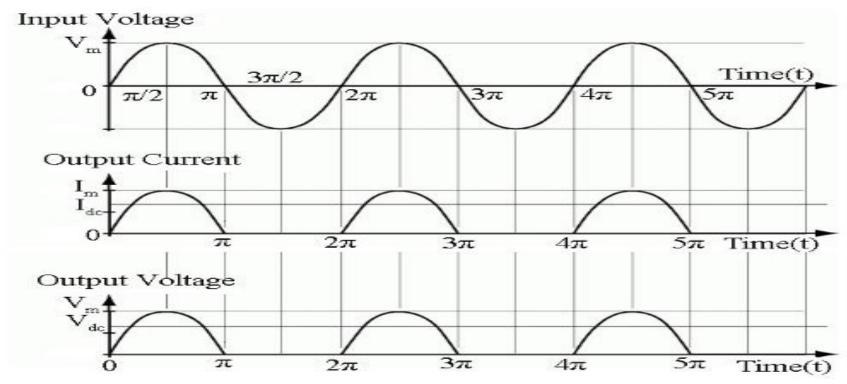
Waveform of Half Wave Rectifier
