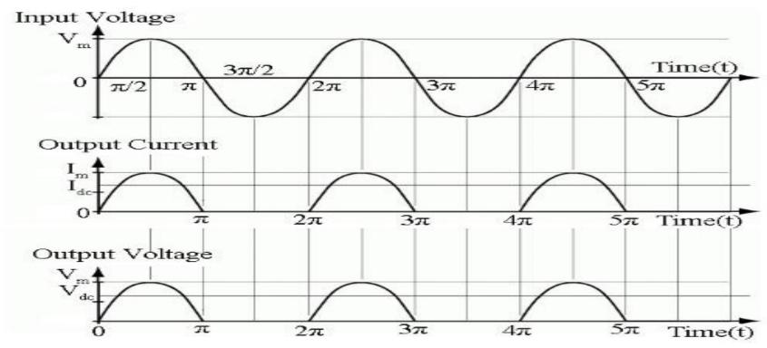
Waveform of Half Wave Rectifier
