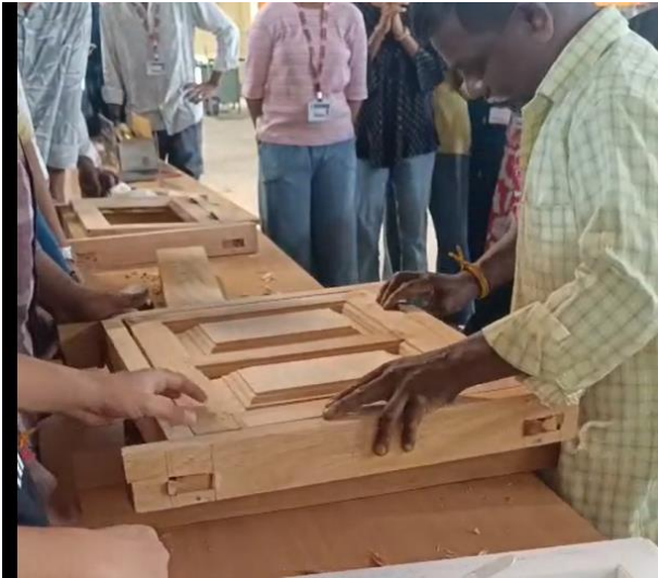
Students assembling wooden door components during Skill Lab-III, learning joinery techniques and precision in carpentry work.
